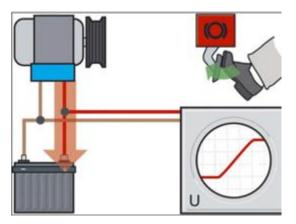
Regenerative Braking systems recover the energy normally converted into and lost as heat during vehicle braking. When available the recovered energy is fed back into the charging system to recharge the battery
