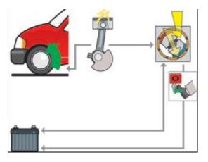
Starter/generator technology replaces the conventional alternator and starter motor with a combined starter/generator unit installed between the engine and the transmission. The vehicle features both Stop/Start and regenerative braking systems that operate in the same way as for Micro hybrid 1 and 2 vehicles but utilises the starter generator for both start/stop and regenerative braking functions.
