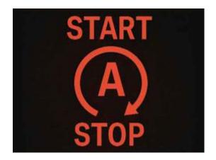
Initially a manual system now becoming fully automatic, switches off the engine when the vehicle is stationary. The engine is restarted automatically by releasing the brake and depressing the accelerator pedal or clutch pedal dependent on transmission type. Initial Stop/Start systems could be manually switched off, but on next generation vehicles this option is disabled
