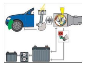
The full hybrid vehicle features a higher power starter generator and an additional clutch between the internal combustion engine and transmission. This allows the decoupling of the engine and starter generator.
