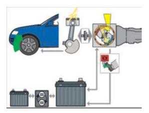
The full hybrid vehicle features a higher power starter generator and an additional clutch between the internal combustion engine and transmission. This allows the decoupling of the engine and starter generator.
