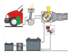
Future new technologies being introduced to the next generation of vehicles include a solution known as "Passive boost". Passive Boost is a simpler more cost effective system related to the Kinetic Energy Recovery System (KERS) recently introduced into the Formula 1 race series
