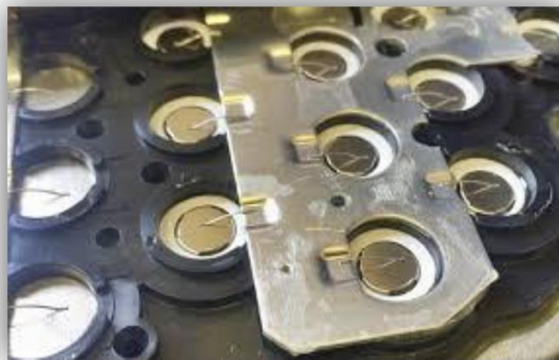
Cells Electrical connection to Bus Bar.
